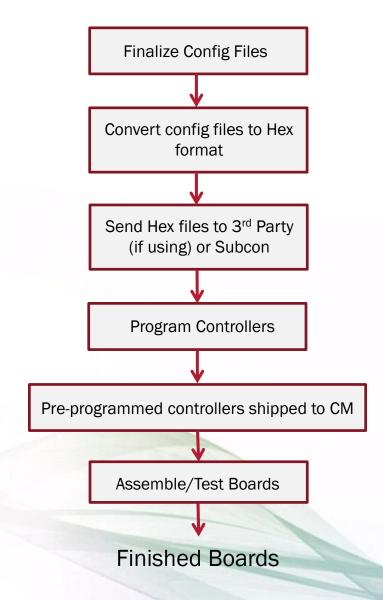
• Controllers are programmed prior to PCB manufacture.
