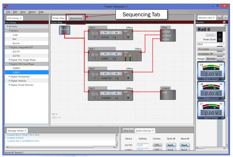
The sequencing tab allows for power up and power down sequencing of devices in the PowerMap.
