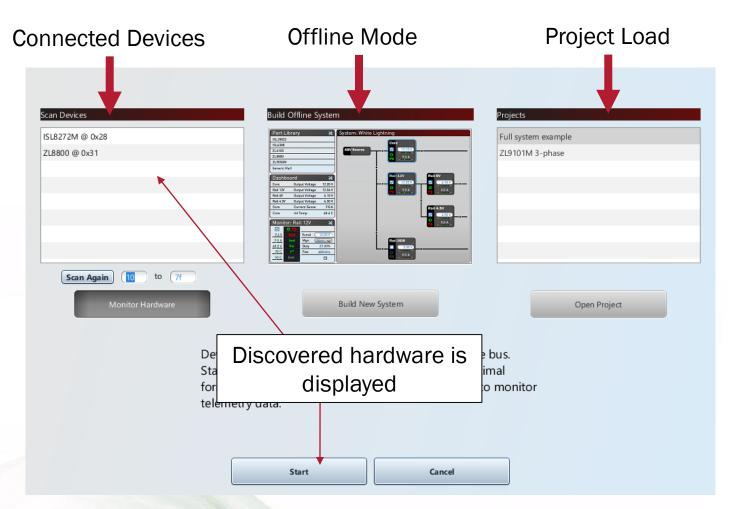
All discovered hardware is displayed in the "Scan Devices" window. The PMBus scan range can be adjust – default range is 0x10 to 0x7F.
