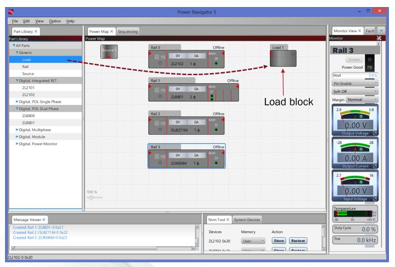
Load Blocks represent system load. Double Click to add additional inputs.
