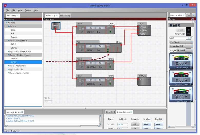
To implement a current sharing rail, drag a part from the part library onto an open RailBlock "slot".
