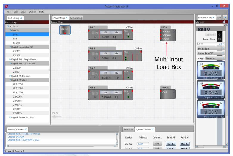
After Configuring system, sources, rails and loads can be wired together.
