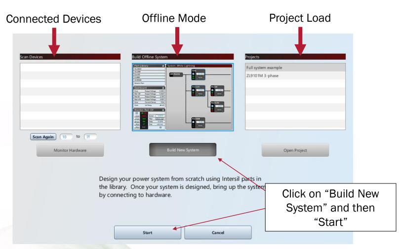
The PowerNavigator launch screen allows you to select online (hardware connected) or offline modes of operation.
